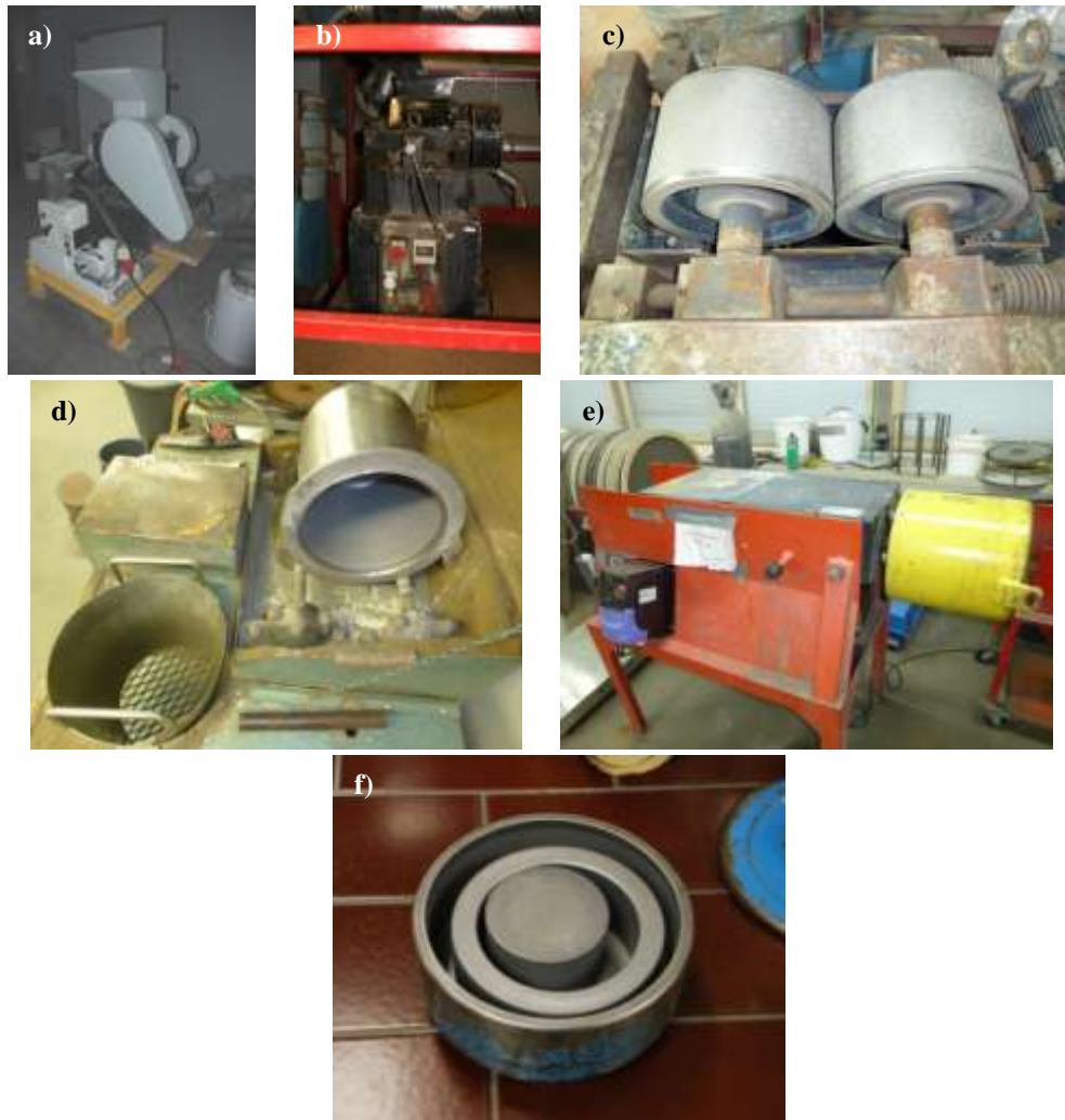
Figure 3: a) Jaw crusher, b) Rolls crusher, c) rolls crusher internal workings, d) Laboratory batch ball/rod mill, e) Mergan rod/ball mill for larger-scale grinding, f) Vibratory disc mill attachment (not attached to machine)
