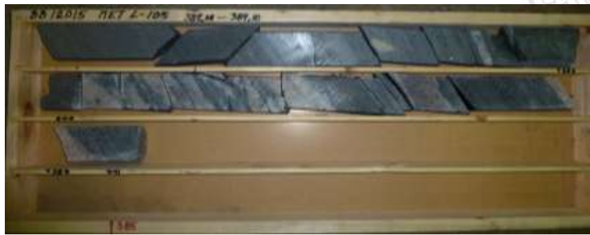
Figure 23: Cores as delivered; 382.08-384.10m (17.9kg)
