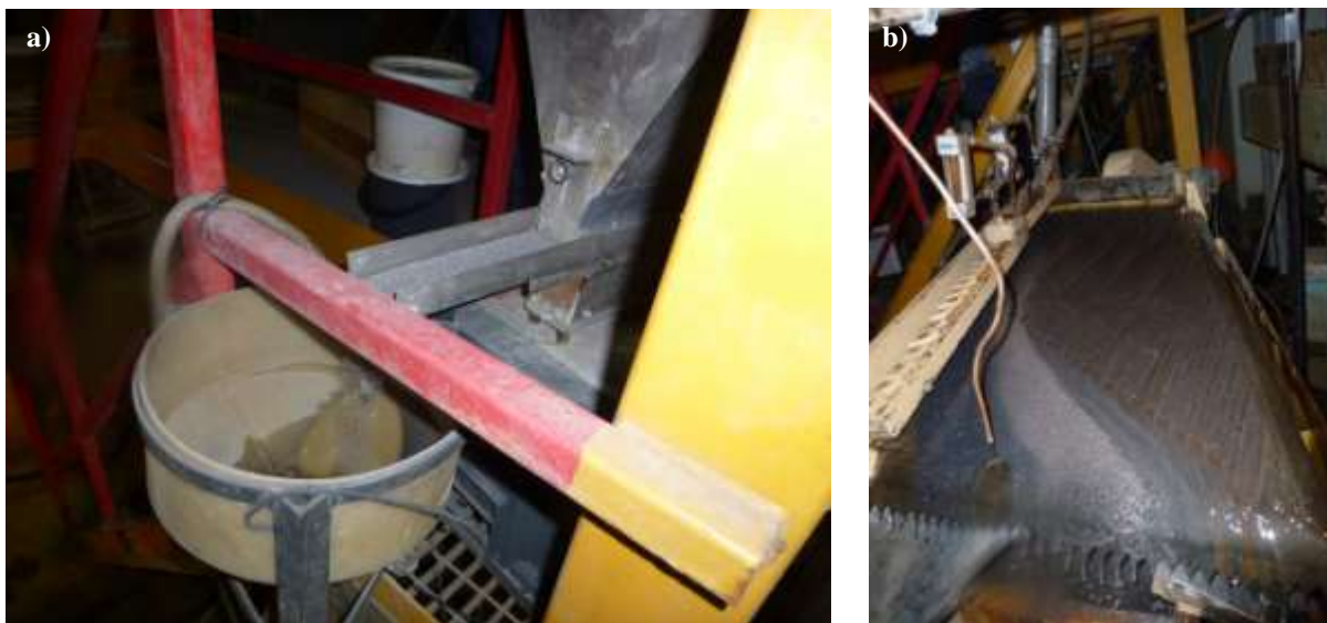
Figure 8: a) Shaking table feed system b) Shaking table
