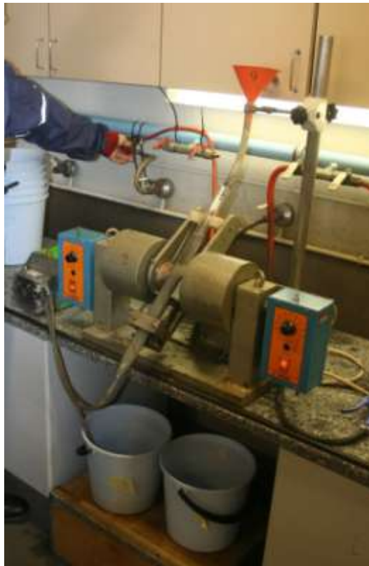
Figure 7: Set-up of Davis Tube equipment
