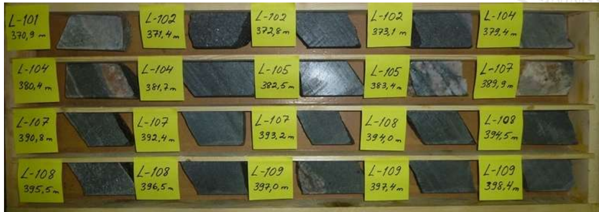
Figure 27: Core samples sent for crushability and abrasion index testing
