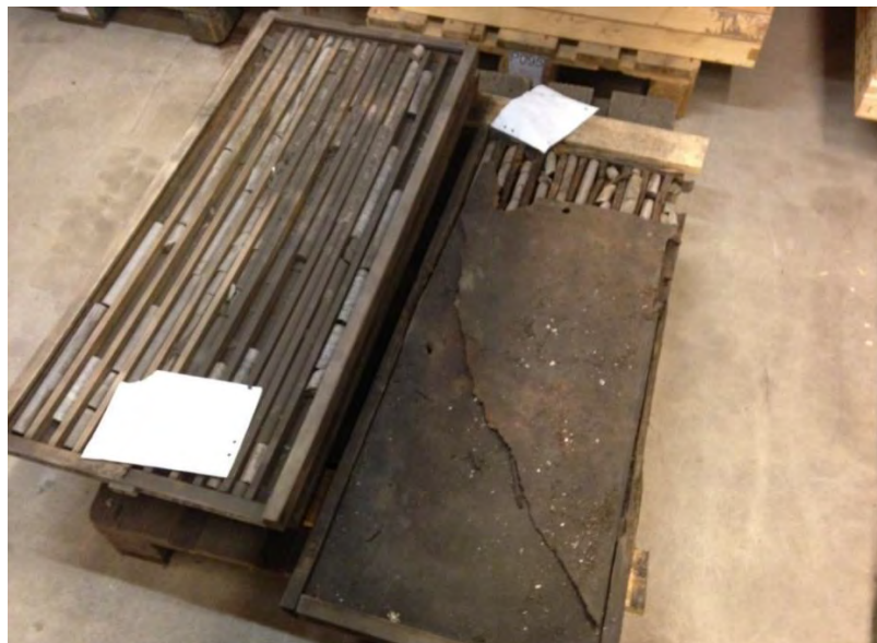
Figure 6-6 Typical condition of recovered historical core and core boxes
